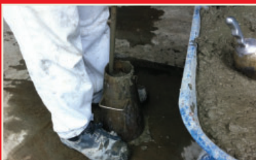
4. Compacting concrete for slump test
